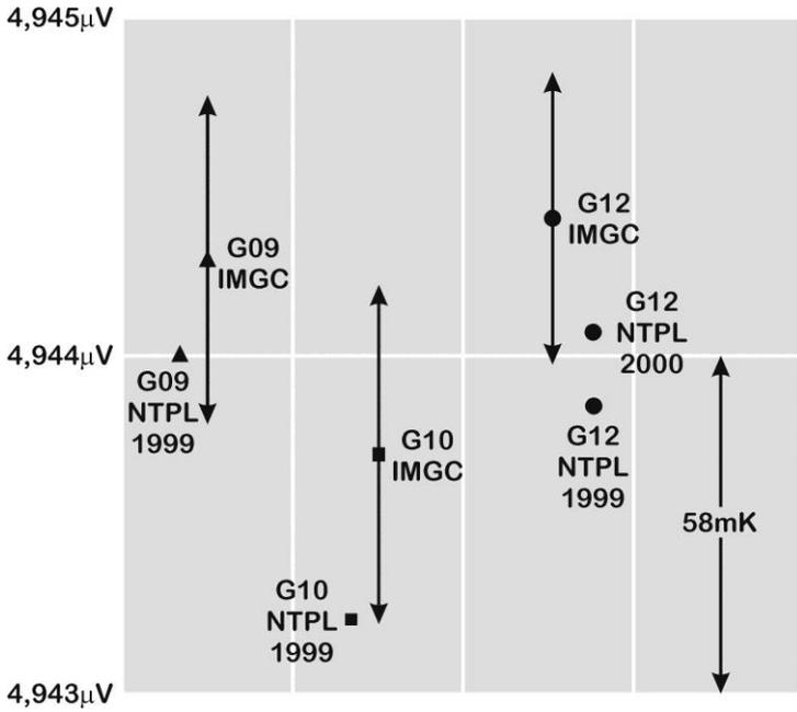
*Gold/Platinum Thermocouple Intercomparison NTPL vs IMGC – Aluminium Point*
