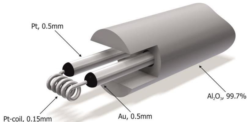
To summarise and simplify their work they found that this thermocouple if made according to their prescription was capable of accuracies of  $\pm 0.02^{\circ}\text{C}$  from  $0^{\circ}\text{C}$  to  $962^{\circ}\text{C}$ .
